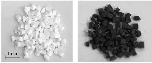
Fig. 1 Alumina support and prepared catalyst.
